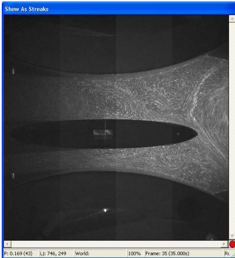
Figure 97: Example image from streaks facility. Here the field of view was 2.5 \times 2.5 m and particles illuminated by a 5W argon laser. The streaks show barotropic vortices interacting with the baroclinic hydraulic exchange through a strait containing an island.
